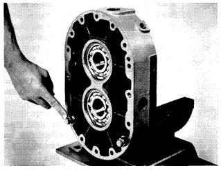
FIGURE 19 TWO CAPSCREWS WITH SPACERS USED TO TEMPORARILY FASTEN DRIVE END PLATE TO LOWER HOUSING HALF.
