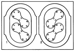
FIGURE 30 POSITIONS OF ROTORS FOR CHECKING TIMING
