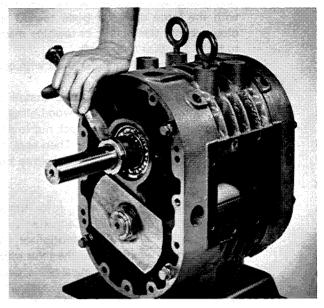
FIGURE 25 TIGHTENING LOCK NUT TO CHECK DRIVE END CLEARANCE
