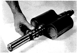
FIGURE 18 ASSEMBLING SHIMS TO DRIVE END OF DRIVE ROTOR SHAFT
