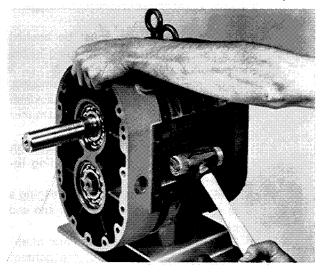
FIGURE 14 USING SOFT FACED MALLET TO LOOSEN DRIVE END PLATE
