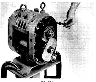
FIGURE 8 FOUR CAPSCREWS WITH SPACERS BEING TEMPORARILY REPLACED IN GEAR END PLATE
