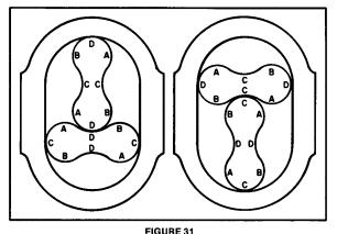
POSITIONS OF ROTORS FOR CHECKING INTERNAL CLEARANCE
