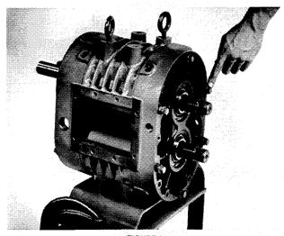
FIGURE 22 SIX CAPSCREWS WITH SPACERS USED TO TEMPORARILY FASTEN GEAR END PLATE TO UPPER AND LOWER HOUSING HALVES
