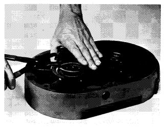
FIGURE 17 INSTALLING RETAINING RING
