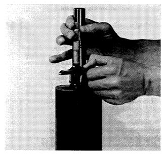
FIGURE 17B MEASURING FROM END OF BEARING SPACER TO END OF ROTOR LOBE
