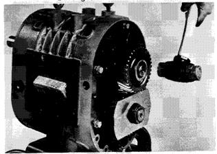
FIGURE 29 STARTING DRIVE GEAR ONTO SHAFT WITH SOFT FACED MALLET
