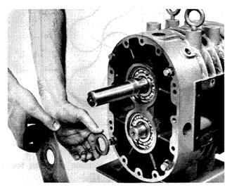
FIGURE 23 ASSEMBLING CLAMP WASHER AND OIL FLINGER TO DRIVE END OF IDLER SHAFT
