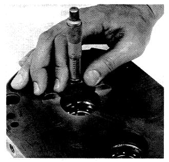
FIGURE 17A MEASURING FROM AIRBOX SURFACE TO INNER RACE OF BALL BEARING
