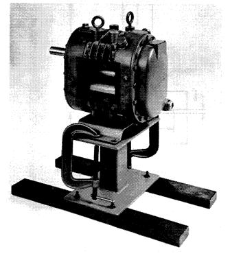
FIGURE 6 BLOWER SECURED TO WORK STAND WITH "C" CLAMPS
