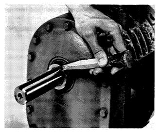
FIGURE 12 USING BLUNTED FLAT CHISEL AND BALL PEEN HAMMER TO LOOSEN LOCK NUT
