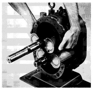
FIGURE 16 REMOVING DRIVE ROTOR FROM GEAR END PLATE
