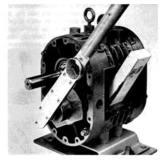
FIGURE 24 TIGHTENING LOCK NUTS WITH TORQUE WRENCH
