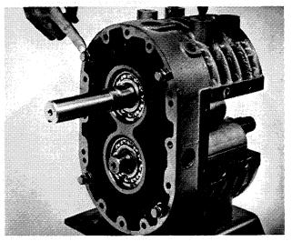
FIGURE 21 TWO CAPSCREWS WITH SPACERS USED TO TEMPORARILY FASTEN UPPER HOUSING HALF TO DRIVE END PLATE
