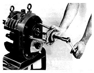
FIGURE 15 USING PULLER TO REMOVE TIMING GEAR
