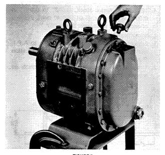
FIGURE 7 REMOVING BREATHER CAPS FROM GEAR END PLATE
