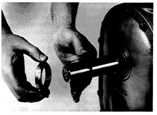
FIGURE 33 ASSEMBLING SPIDER WASHER AND LOCK NUT TO DRIVE SHAFT
