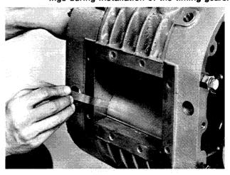
FIGURE 28 CHECKING DRIVE END CLEARANCE WITH FEELER GAGE
