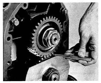
FIGURE 10 INDEX MARKS ON ENDS OF GEAR TEETH
