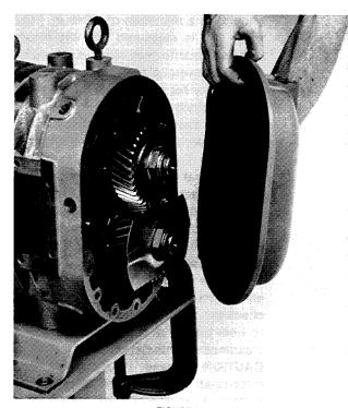
FIGURE 32 ASSEMBLING GEAR END COVER AND GASKET TO END PLATE
