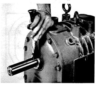
FIGURE 34 TIGHTENING DRIVE SHAFT LOCK NUT SECURELY WITH BLUNTED CHISEL AND BALL PEEN HAMMER
