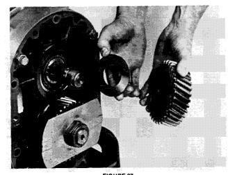
FIGURE 27 POSITIONING BELLEVILLE SPRING AND DRIVE GEAR BEFORE ASSEMBLING TO DRIVE ROTOR SHAFT
