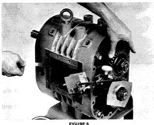
FIGURE 9 CHECKING TIMING GEAR BACKLASH WITH DIAL INDICATOR
