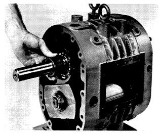
FIGURE 13 REMOVING BEARING SPACER FROM DRIVE SHAFT
