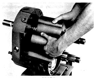
FIGURE 20 ASSEMBLING DRIVE ROTOR TO DRIVE END PLATE
