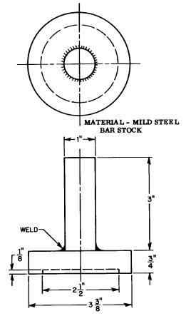
FIGURE 5 BEARING INSTALLATION TOOL
