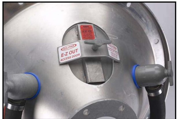
Easy Out Access Door on bulk trailer bottom
